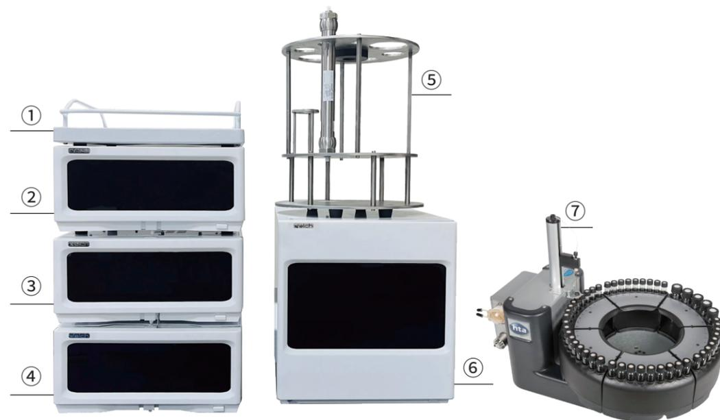
Schematic diagram of WelPrep2000 preparative liquid chromatography instrument
