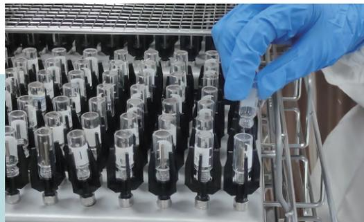
2. During the cleaning process of sample vials, a specially designed basket rack is used, with each sample vial having a dedicated cleaning nozzle. This ensures that the incoming water effectively flushes out any contaminants. The outer surface of the vials is subjected to a circulating rinse using upper and lower spray arms, enabling a 360-degree cleaning of the sample vials. This ensures that even hard-to-clean sample vials are thoroughly cleaned.
